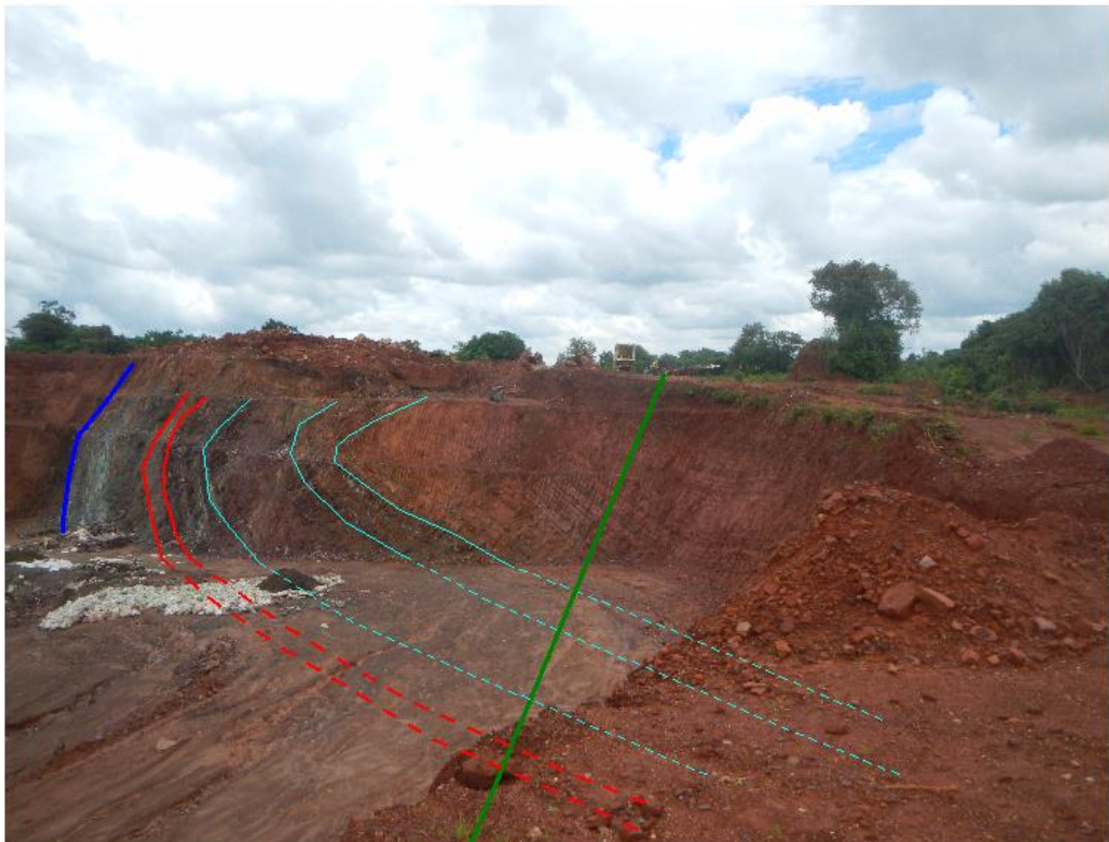
Figure 3; Kasombo 5 Prospect Drillhole KSB001; projection of drillhole shown with the dark green line, and bedding layers drawn on the pit-wall of the open cut; image of pit showing bedding (with light blue line, down-dip projection as dotted line); basal fault (dark blue line); mineralisation target (red lines, down-dip projection as dotted line); drill rig in position (but with its mast down) outside the rim of the pit.
